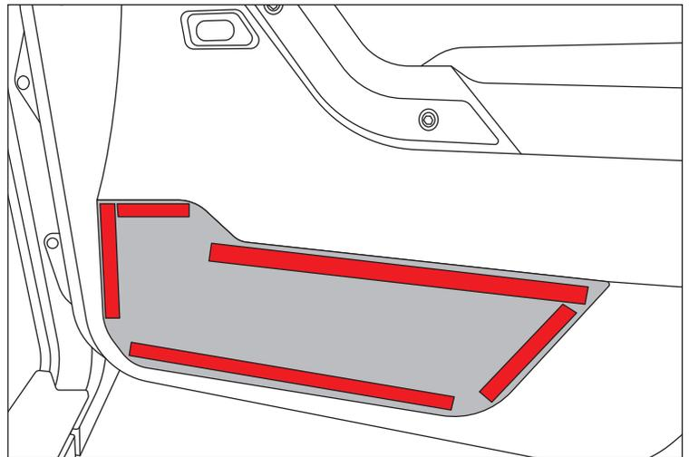
3. Remove backing of hook and loop strip and install on vehicle in area shown. Press and hold firmly for 30 seconds to ensure proper adhesion. Do not use door storage panels for first 24 hours to ensure proper adhesion. Repeat steps 2-3 for opposite side.
