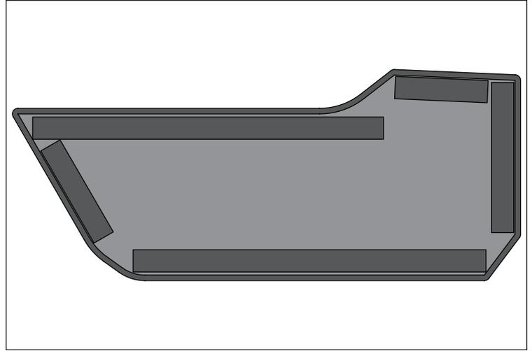
2. Clean lower area of door panel with isopropyl alcohol and apply adhesion promoter where hook and loop strips will tape to door. Allow 90 seconds for adhesion promoter to properly dry before continuing.
